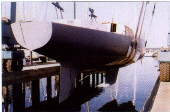
Figure 3 —The author designed a new keel for Zanabe , a 25-year-old 72' (22m) wooden sloop. The keelbolts were L-shaped stainless steel rods, "caged" to lock them into the casting. Left — Zanabe 's keel installed. This is a fairly traditional low-aspect-ratio design, and includes a beavertail bulb that keeps weight low and reduces the tip vortex flowing off the lower end of the keel's trailing edge.
